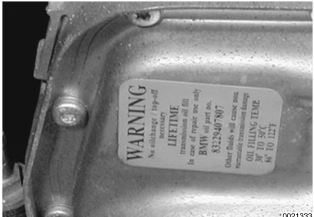
► The automatic transmissions installed in the 3 Series are filled with a number of different transmission fluids. Each transmission should have a colored label on the ATF sump identifying the fluid type installed..
